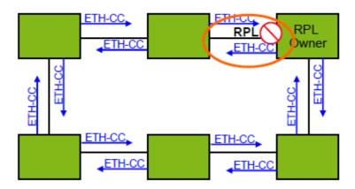
When a node on the link detects a fault, it immediately blocks the faulty node and reports the fault message (R-APS (SF)) to all the other devices in the ring. After receiving the message, all other nodes refresh the FDB. The RPL owner port receives the fault message, and the recovery port is in the forwarding state. The ERPS ring enters the protection state. As shown in the Figure:
