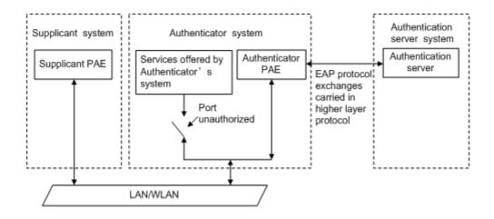
The above systems involve three basic concepts: PAE, controlled port, control direction.
