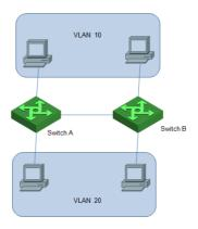
A VLAN can span across multiple GPONes, or even routers. This enables hosts in a VLAN to be dispersed in a looser way. That is, hosts in a VLAN can belong to different physical network segment.
