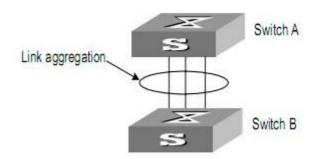
For the member ports in an aggregation group, their basic configuration must be the same. The basic configuration includes STP, QoS, VLAN, port attributes, and other associated settings.
