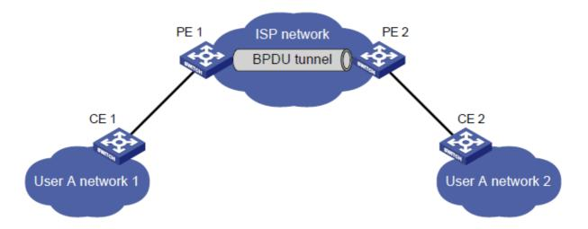
With L2TP, Layer 2 protocol packets from customer networks can be transparently transmitted in the service provider network:
