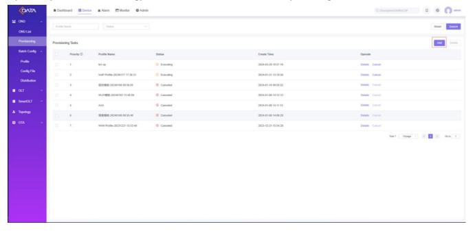
Select the configuration profile and the configuration object. The configuration object can match the device according to the vendor, model or SN. If multiple items are entered, the intersection match will be taken. If neither of these parameters is specified, there is no limit. The profile will be automatically delivered to any device reported for the first time.
