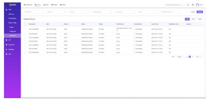
Click Add to create a batch configuration task, select the configuration profile and object, and deliver the task directly.
