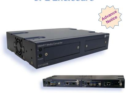
The CH1202B is a CPE enclosure that supports two MC2700B series media converter modules. This enclosure is both wall mountable as well as 19" 1RU rack mountable. Two CH1202B chassis can be mated together using strong ties and fit in a 19" 1RU space to support up to four MC2700B series media converter modules. This enclosure also supports redundant (load sharing) 5V DC powering with LED indicators and "dying gasp" capability.
