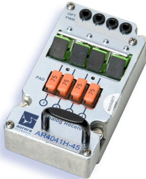
The AR4041 series Analog Quad Return Path Receivers (RPRs) are designed as plug-in modules for Aurora's NC4000 optical nodes. These receivers are available for low or high RF gain (for corresponding optical input ranges of  $-7$  to  $+3$  dBm, or  $-15$  to  $-7$  dBm, respectively) for both 5–45 or 5–65 MHz passbands. Their compact design (single-width module) makes them the highest density packaging RPRs available.
