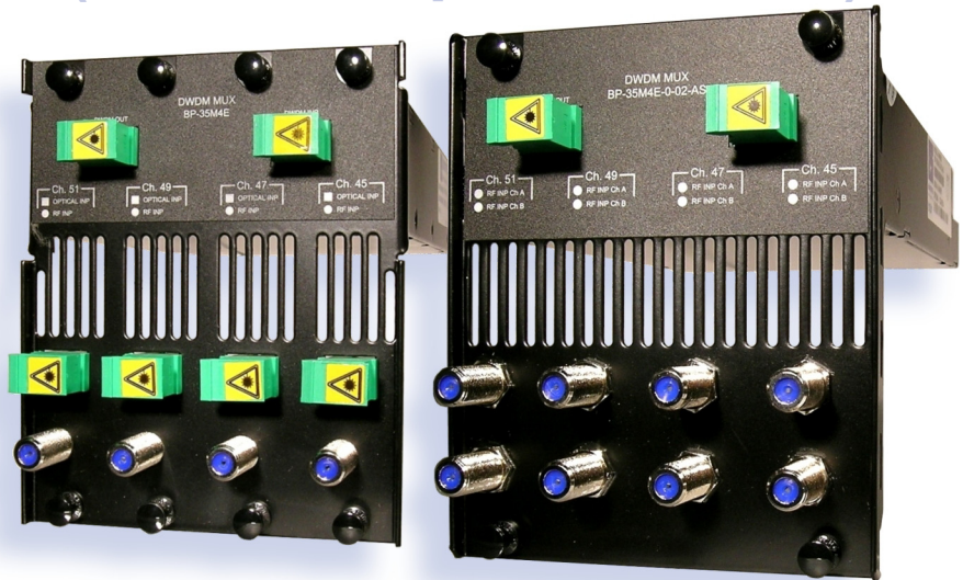
Two representative models of BP-35M4x series Optical Mux Back Plates: BP-35M4x-1-00-AS (used with AT3510 Analog Narrowcast Transmitters or DX3515 Digital Transponders) and BP-35M4x-1-02-AS (used with DT3515 Return Path Digital Transmitters)
