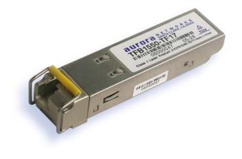
The TFB1550-TF17 Bi-Directional Optical Transceiver Module is ideally suited for Fast Ethernet and PON applications where a single fiber is required to simultaneously carry both Tx and Rx signals up to 20 km (over SMF). The built-in high isolation WDM enables full duplex operation.
