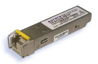
The TFA1310-TF17 Bi-Directional Optical Transceiver Module is ideally suited for Fast Ethernet and applications where a single fiber is required to simultaneously carry both Tx and Rx signals up to 20 km (over SMF). The built-in high isolation WDM enables full duplex operation.
