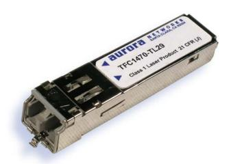
TFCxxxx-TL29 series CWDM Optical Transceiver Modules are ideally suited for Fast Ethernet applications. Conforming to the Small Form Factor Pluggable (SFP) Multisource Agreement, these state-of-the-art plug-in components are designed for applications that require rates of up to 125 Mbps, with the laser transmission portion of the device operating at one of 10 available ITU-compliant (G.694.2) CWDM wavelengths. The modules are supplied with a duplex LC connector.
