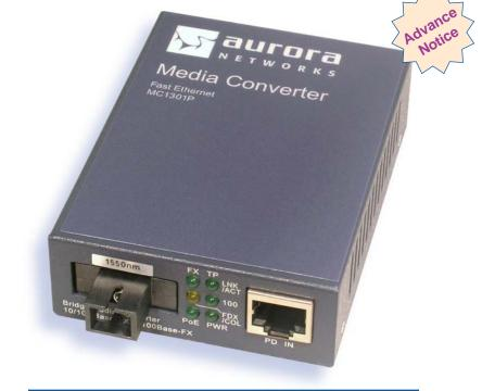
Aurora Networks' MC1301P-1550-SF Media Converter is compliant with the IEEE 802.3af Power over Ethernet standard and permits network planners to connect 10 or 100 Mbps twisted pair network segments to single-mode or multi-mode fiber optic access networks. It receives 10/100 Mbps data and power from an external PSE or PoE injector through its PD IN port and functions as a 10/100Base-TX to 100Base-FX media converter.
