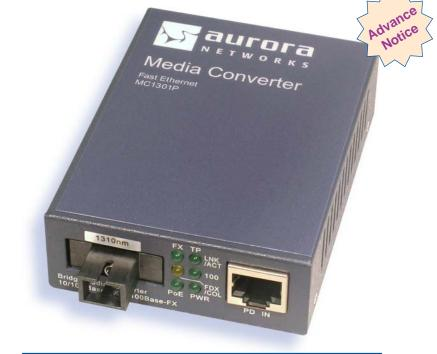
Aurora Networks' MC1301P-1310-SF Media Converter is compliant with the IEEE 802.3af Power over Ethernet standard and permits network planners to connect 10 or 100 Mbps twisted pair network segments to single-mode or multi-mode fiber optic access networks. It receives 10/100 Mbps data and power from an external PSE or PoE injector through its PD IN port and functions as a 10/100Base-TX to 100Base-FX media converter.
