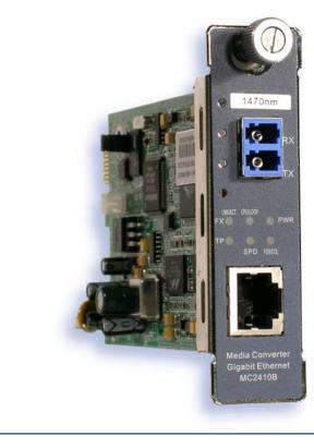
Aurora Networks' MC2410B series GbE SMART Media Converter modules enable network planners to connect 1000 Mbps twisted pair network segments to single-mode fiber optic access networks.
